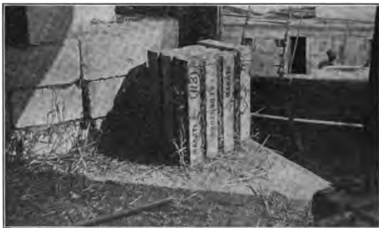
FIG. 151.—Special firebrick shapes crated for export; package 16 in. \times 22 in. \times 32 in. packed in straw, cleats 3 1/2 in. \times 3/4 in., wired; very good packing. Large pieces of regular shape were shipped loose as shown.
